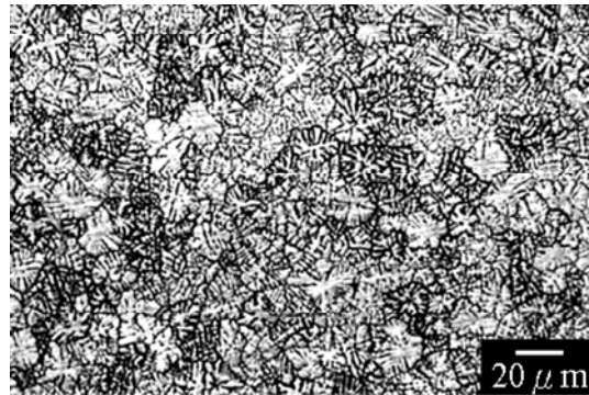
Fig .1. Optical micrograph of the as cast alloy exhibits the dendritic structure.
